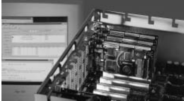
PCI Server during system validation with the Agilent E2928A
