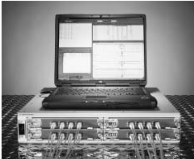
The Agilent 1730 Series SAN test system ensures that the components in a Fibre Channel SAN solution work together properly.
