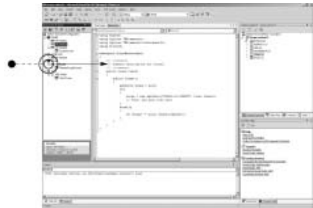
Figure 1. Drag and drop capability saves you programming time and effort. Just drop an instrument icon into your work window to generate code to talk to the instrument.
