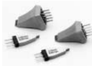
3- and 8-signal versions for 0.5 and 0.65 mm IC Packages.
