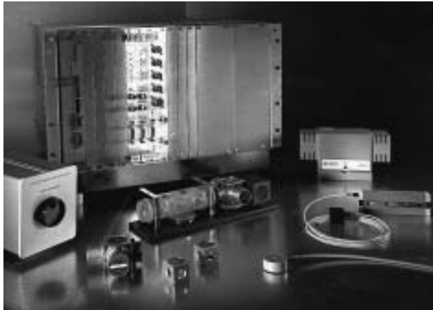
The 10897B High Resolution Laser Axis Board for VMEbus provides the highest position resolution available from Agilent and allows easy, cost-effective integration into this popular, 32-bit industry-standard backplane.
