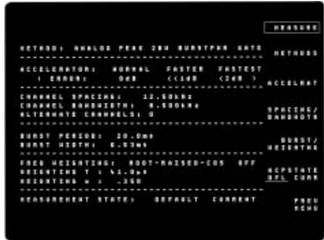
Setup menu for adjacent channel power measurements
