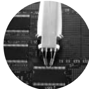
InfiniiumMax 6 GHz differential browser probe head.
